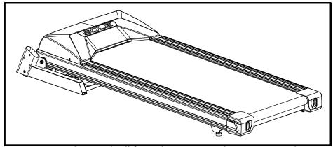
Remove the treadmill from the carton and position it aside on a smooth, level floor. The rear should be at least 3' from any wall. Do not remove the Velcro belt until you have removed the plastic wrap and Styrofoam from beneath the unit. Turning the unit on its side after removing the belt may cause the unit fold up and cause serious injury!
