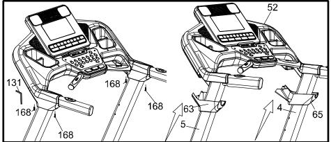
Attach the Left (63) and Right (65) Lower Handlebar Covers to the console with four Sheet Metal Screws (168). Tighten with the Combination M5 Allen Wrench & Phillips Head Screw Driver (131).
