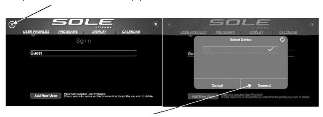
After the equipment is detected, tap Connect. When the App and equipment are synced, the Bluetooth® icon on the equipment's console will light up. You may now start using your new Sole product!
