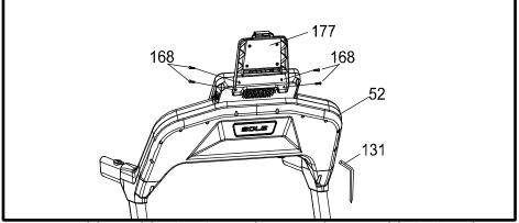
1. Insert Tablet Holder (177) into the Console Assembly (52) and use Combination M5 Allen Wrench & Phillips Head Screw Drive (131) to tighten four of Sheet Metal Screw (168).
