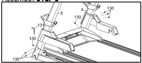
Attach the Upright Tubes (4 & 5) onto the Frame Base (2) with eight Button Head Socket Bolts (130) by using the Combination M5 Allen Wrench & Phillips Head Screw Driver (131). Do not tighten the bolts completely until Step 7 is finished.
