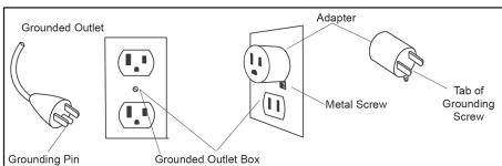
cover. Whenever the adapter is used, it must be held in place by a metal screw.
